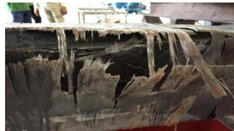
Fig. 3: Strengthening Pattern and Failure of WF90°
