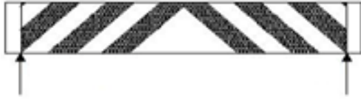
Fig. 5: Strengthening Pattern and Failure of V45°
