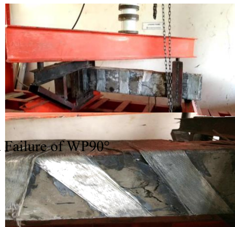
Fig. 3: Strengthening Pattern and Failure of WF90°
