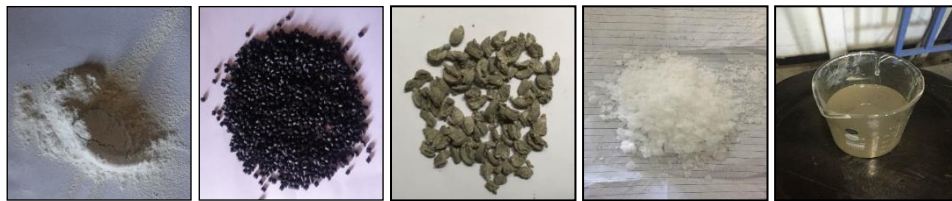
(a) PVC Powder (b) HDP Granules (c)RPA Granules (d)NaOH Pellets (e) \text{Na}_2\text{SiO}_3
