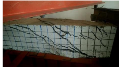
Fig. 2: Strengthening Pattern and Failure of N1
