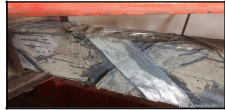
Fig. 6: Strengthening Pattern and Failure of X45°
